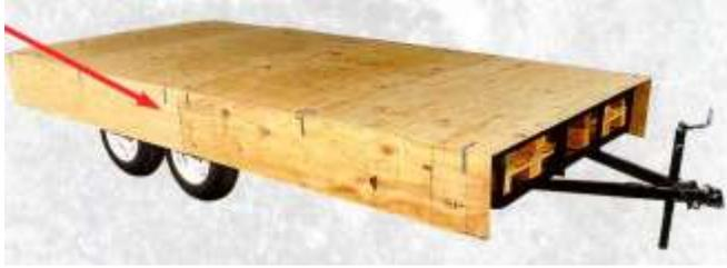
can be used to fasten the skirt frame to the rails: U-shaped brackets are ideal for attachment of the skirt frame to the trailer bed rails. Be sure to terminate the skirt frame approximately 16" from the ground and allow for tongue movement at the front of the float.
